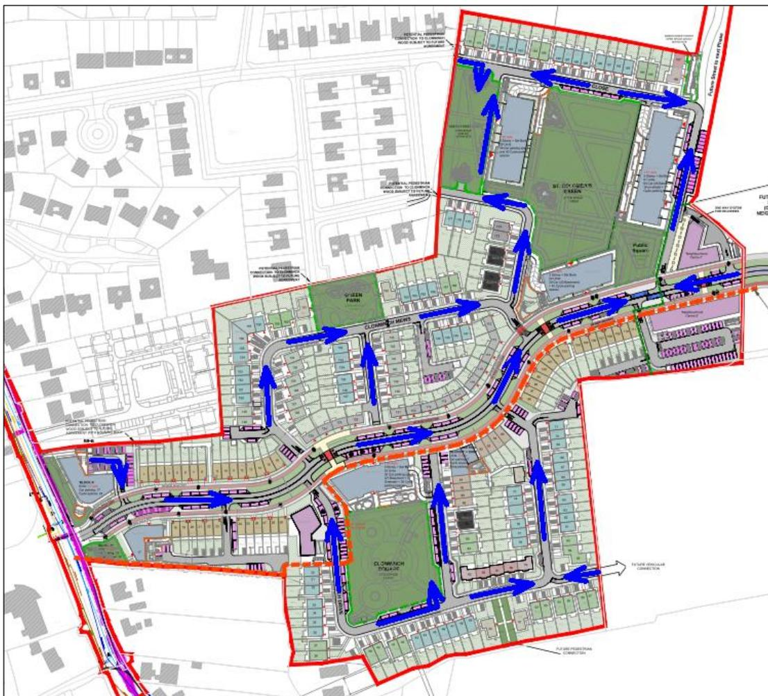
**Figure 5.1 – Flood Exceedance (>1%AEP) Overland Flow Routes**
