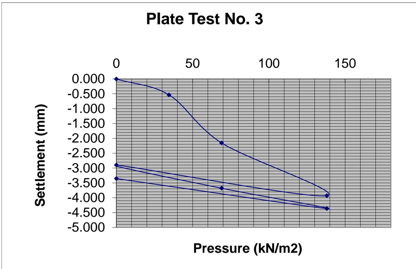
Modulus of subgrade reaction, K (Initial) = **21.63 MN/m<sup>2</sup>/m**
