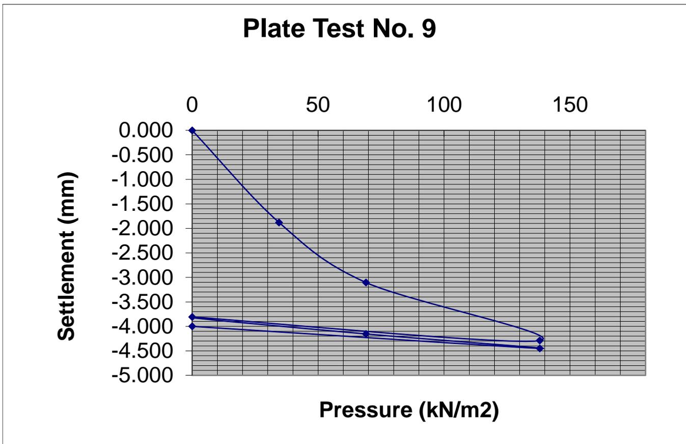
Modulus of subgrade reaction, K (Initial) = **15.02 MN/m<sup>2</sup>/m**
