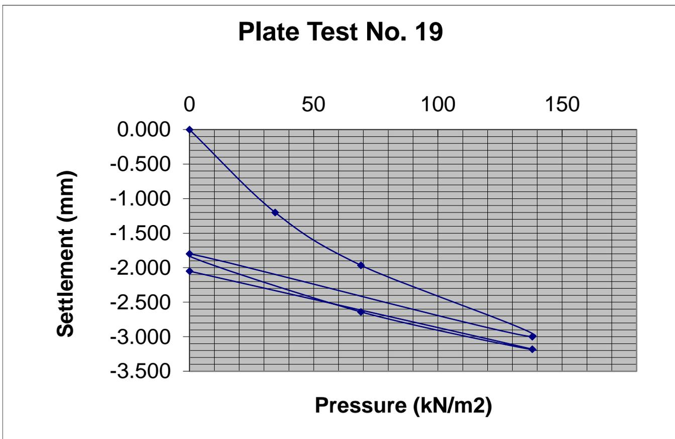
Modulus of subgrade reaction, K (Initial) = **23.73 MN/m<sup>2</sup>/m**
