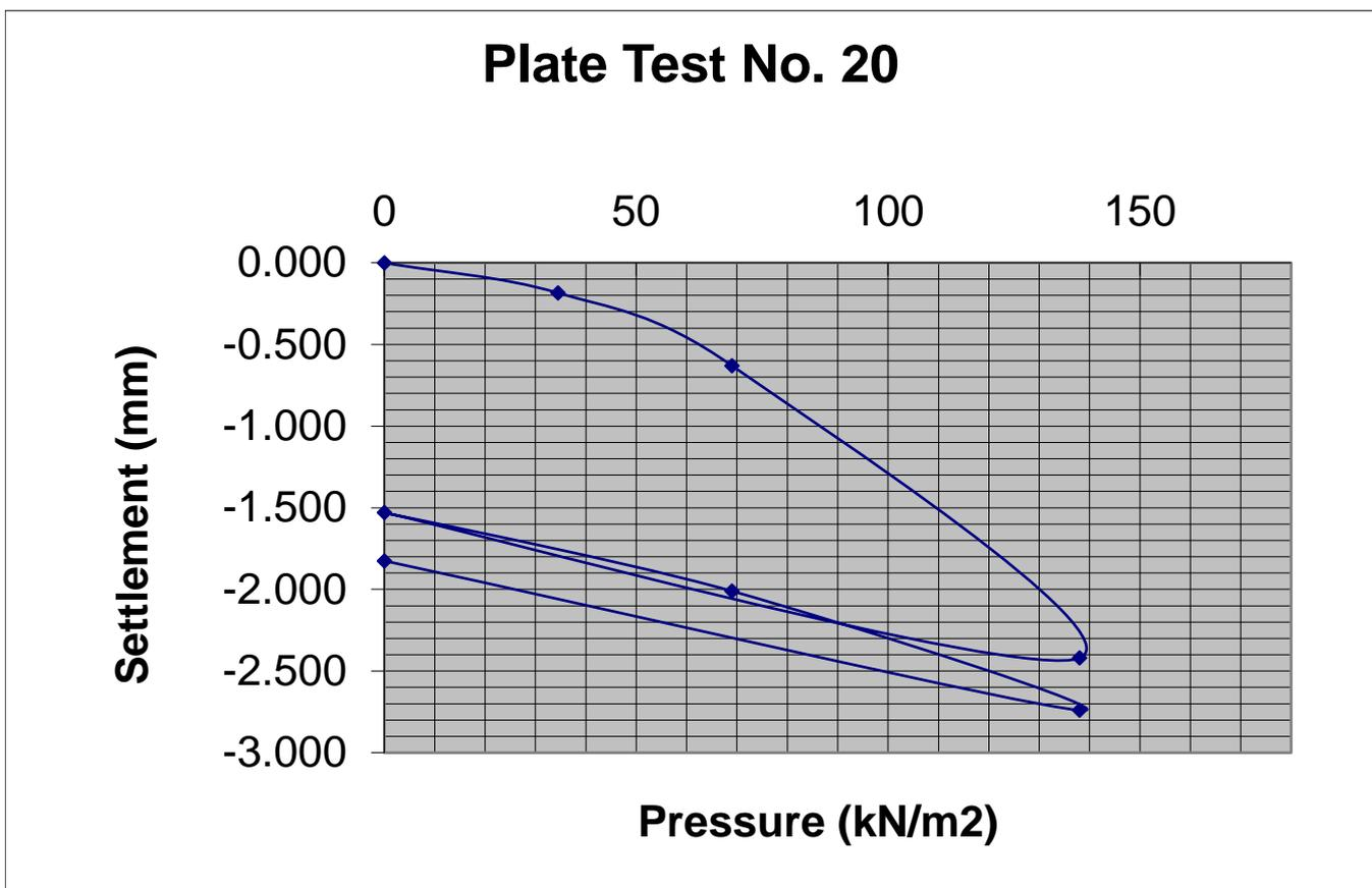
Modulus of subgrade reaction, K (Initial) = **74.01 MN/m<sup>2</sup>/m**
