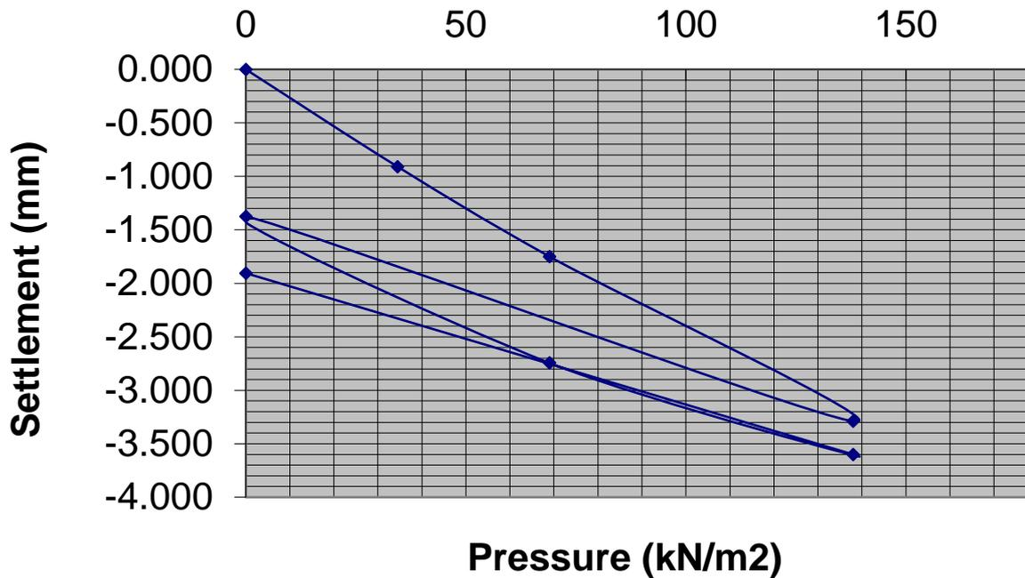
Modulus of subgrade reaction, K (Initial) = **26.64 MN/m<sup>2</sup>/m**
