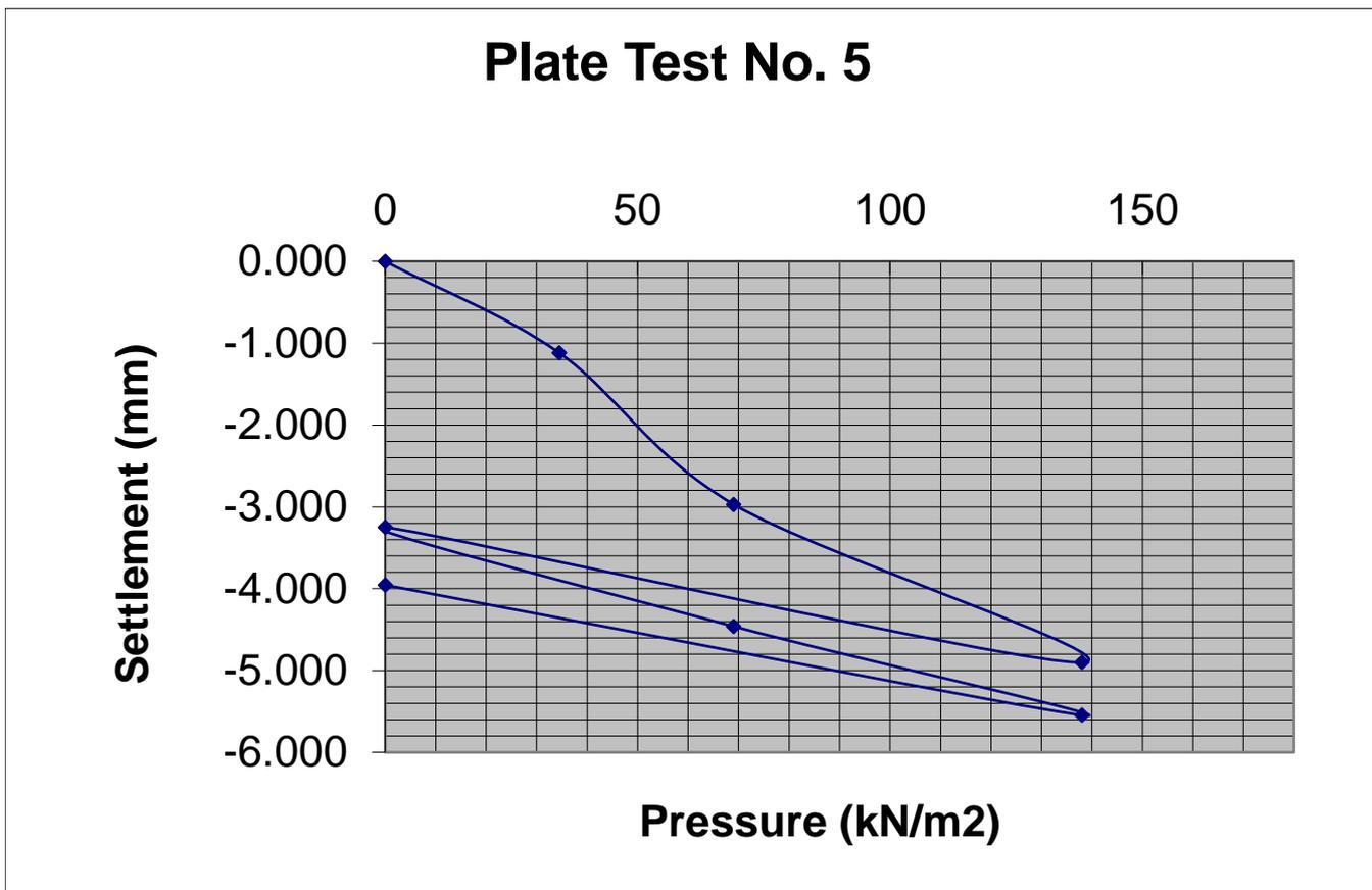
Modulus of subgrade reaction, K (Initial) = **15.70 MN/m<sup>2</sup>/m**
