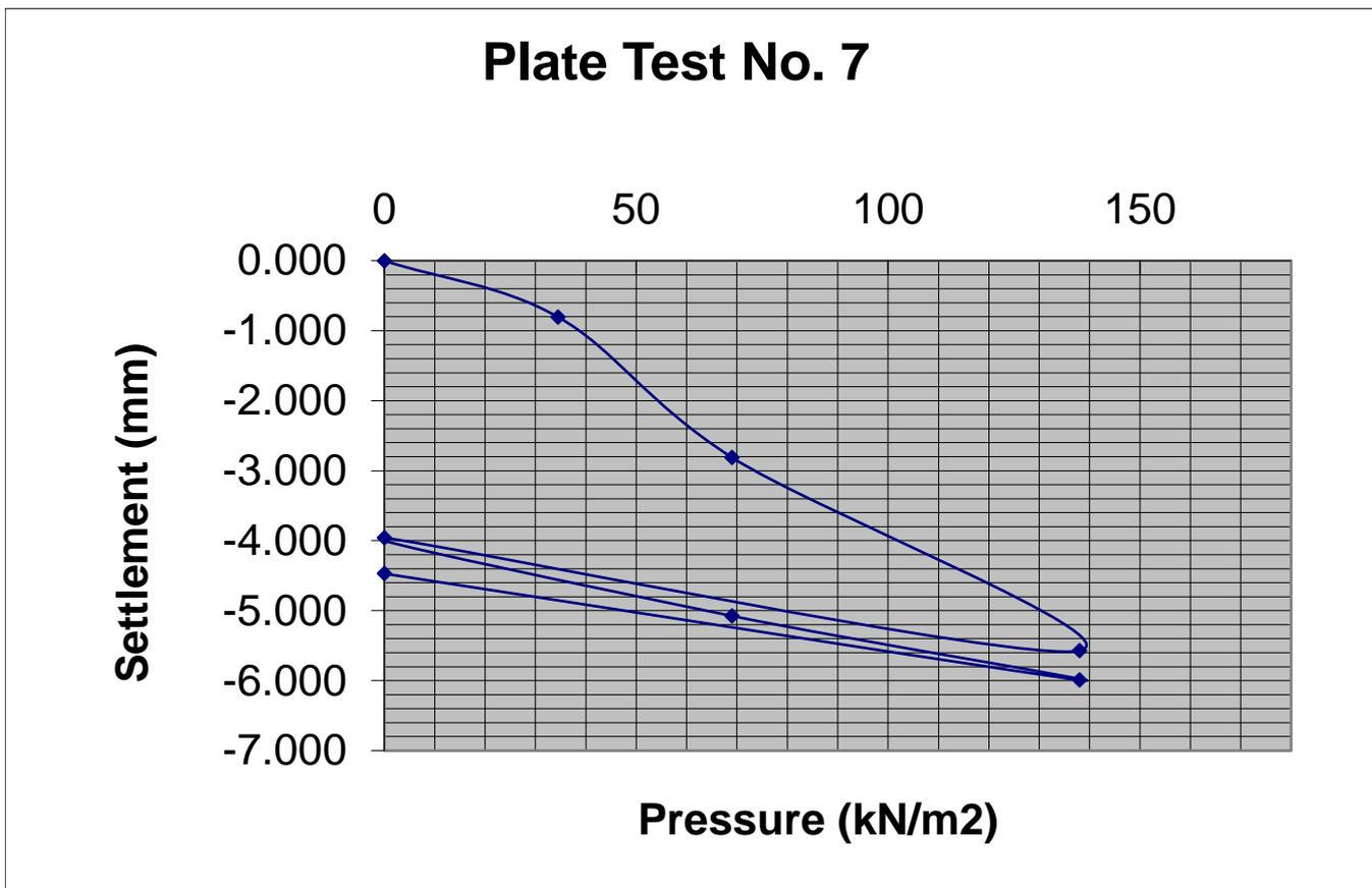
Modulus of subgrade reaction, K (Initial) = **16.59 MN/m<sup>2</sup>/m**
