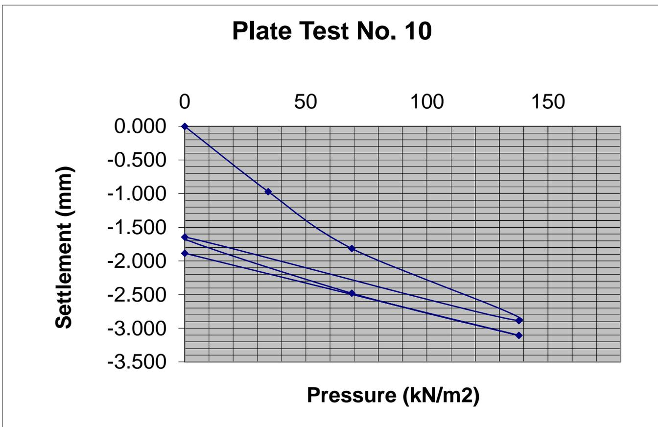
Modulus of subgrade reaction, K (Initial) = **25.69 MN/m<sup>2</sup>/m**
