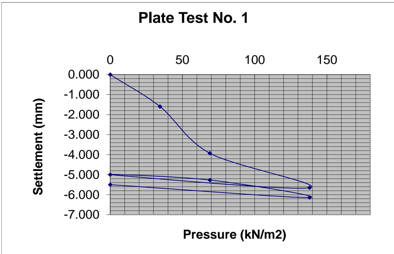
Modulus of subgrade reaction, K (Initial) = **11.86 MN/m<sup>2</sup>/m**
