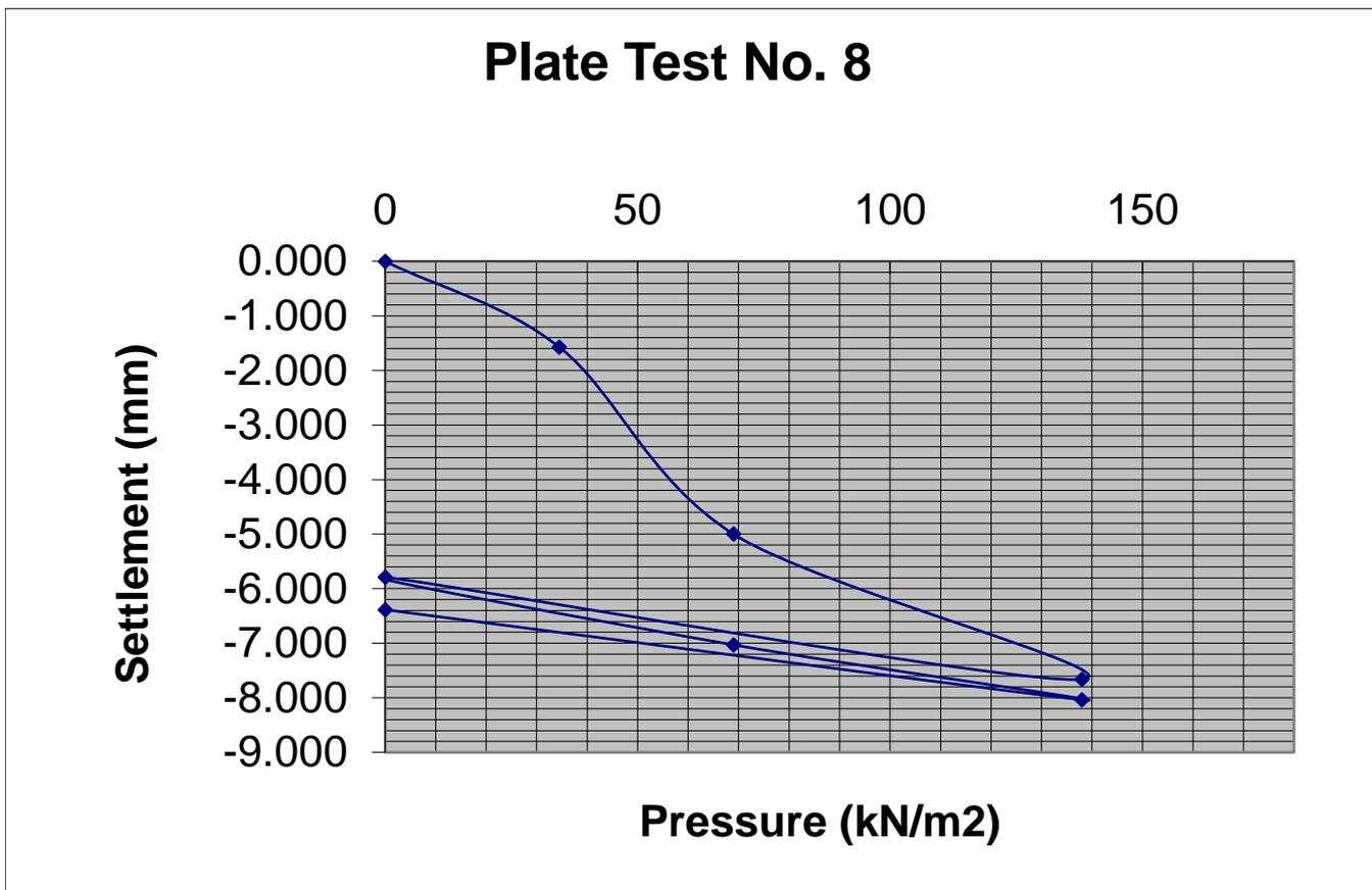
Modulus of subgrade reaction, K (Initial) = **9.32 MN/m<sup>2</sup>/m**
