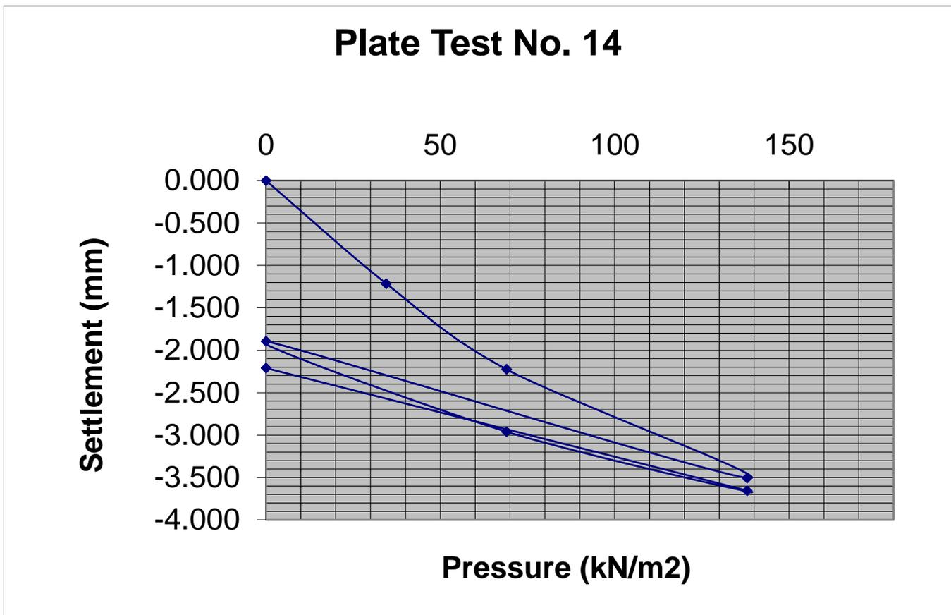
Modulus of subgrade reaction, K (Initial) = **20.95 MN/m<sup>2</sup>/m**
