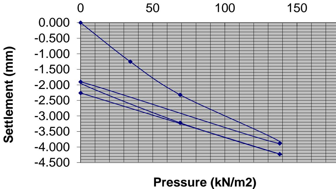
Modulus of subgrade reaction, K (Initial) = **20.10 MN/m<sup>2</sup>/m**
