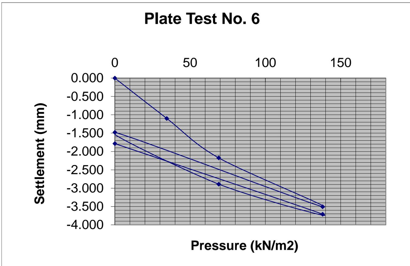
Modulus of subgrade reaction, K (Initial) = **21.44 MN/m<sup>2</sup>/m**
