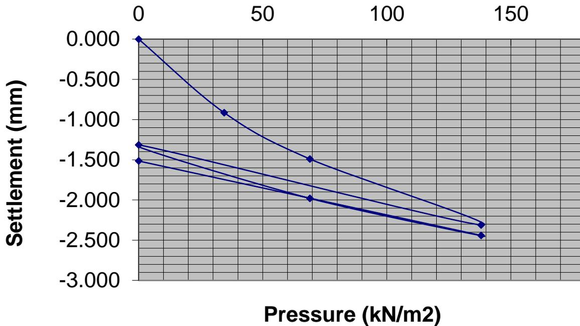
Modulus of subgrade reaction, K (Initial) = **31.29 MN/m<sup>2</sup>/m**
