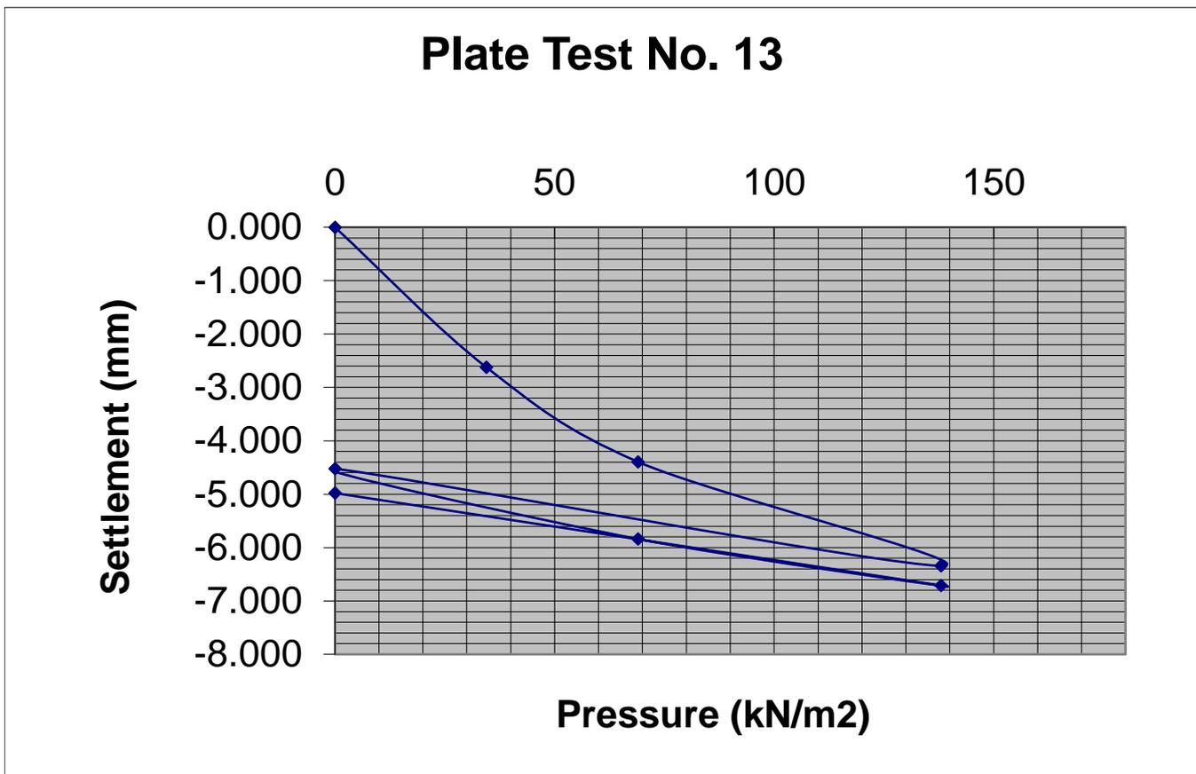
Modulus of subgrade reaction, K (Initial) = **10.61 MN/m<sup>2</sup>/m**
