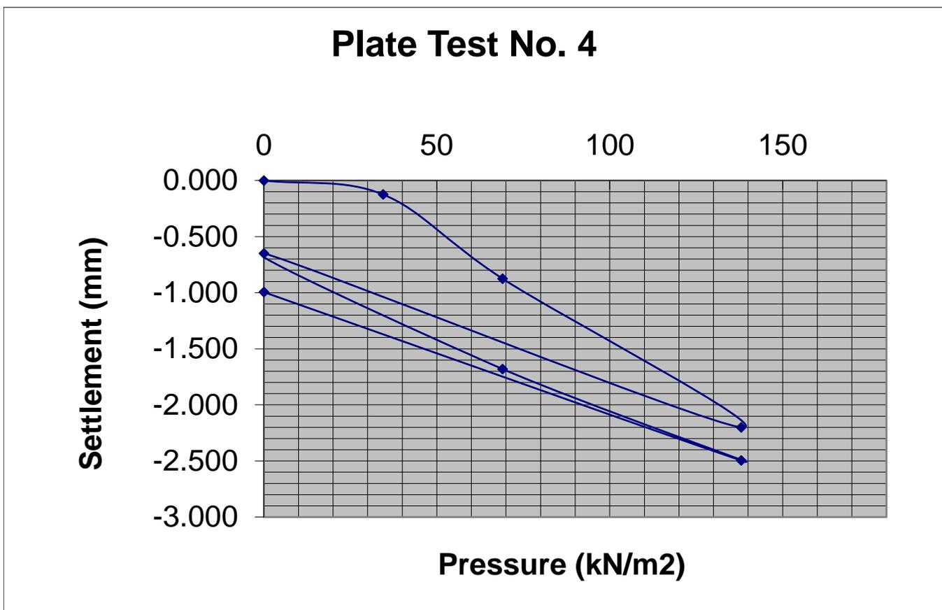
Modulus of subgrade reaction, K (Initial) = **53.28 MN/m<sup>2</sup>/m**
