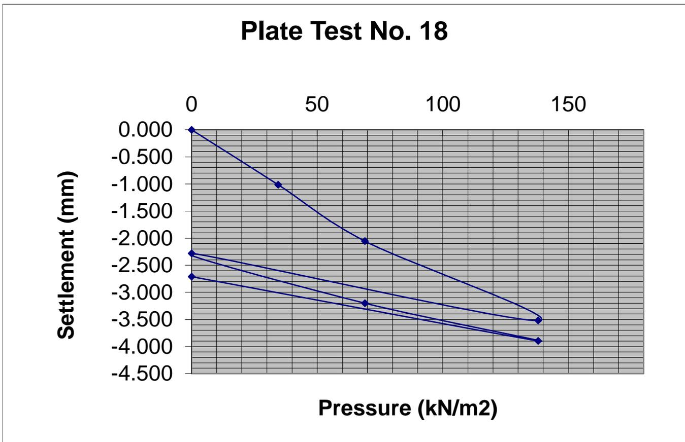
Modulus of subgrade reaction, K (Initial) = **22.69 MN/m<sup>2</sup>/m**
