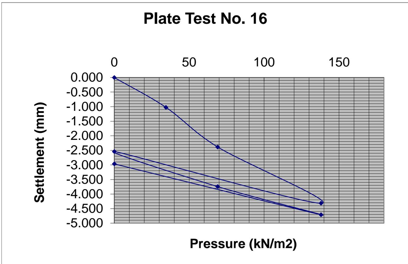
Modulus of subgrade reaction, K (Initial) = **19.55 MN/m<sup>2</sup>/m**
