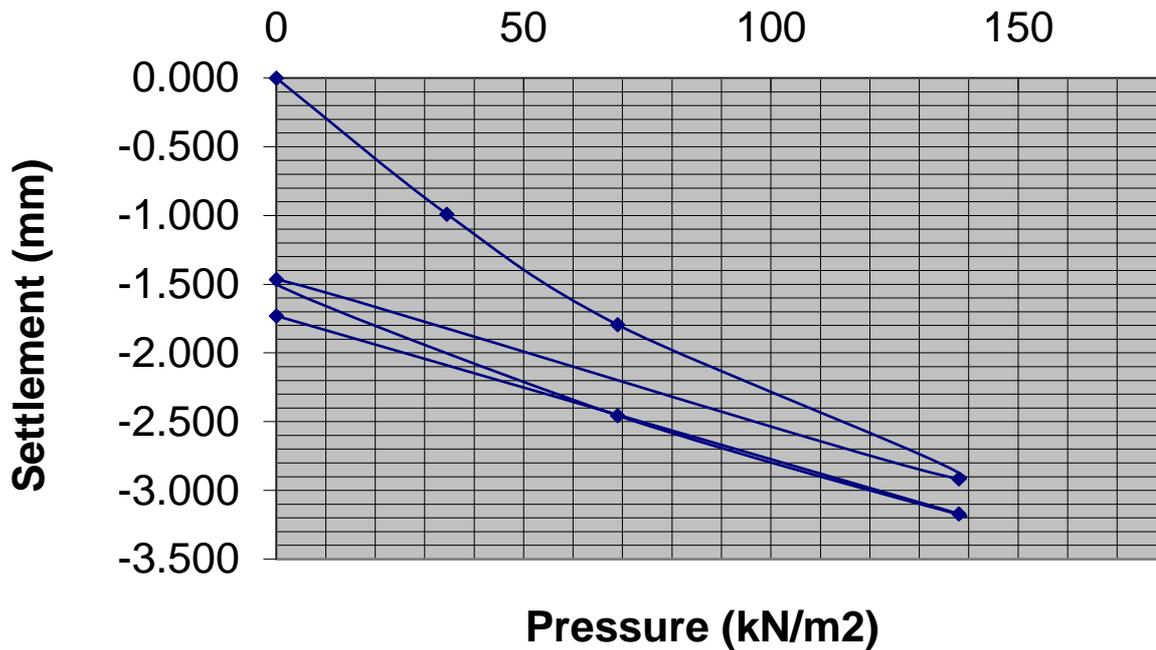
Modulus of subgrade reaction, K (Initial) = **25.97 MN/m<sup>2</sup>/m**
