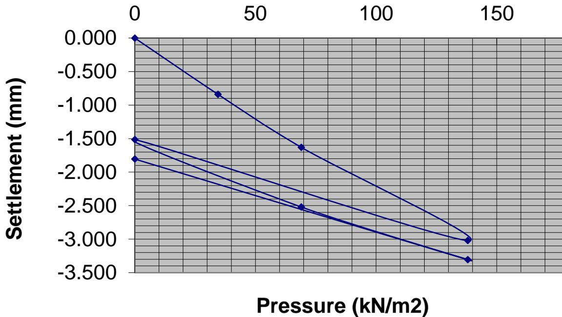
Modulus of subgrade reaction, K (Initial) = **28.60 MN/m<sup>2</sup>/m**
