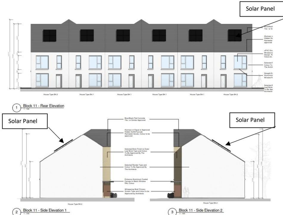
Figure 2: Extract from drawing no. 1757-PA-202 Block 11 demonstrating house design addressing link street – three storey fronting link street and two storey to the rear.
