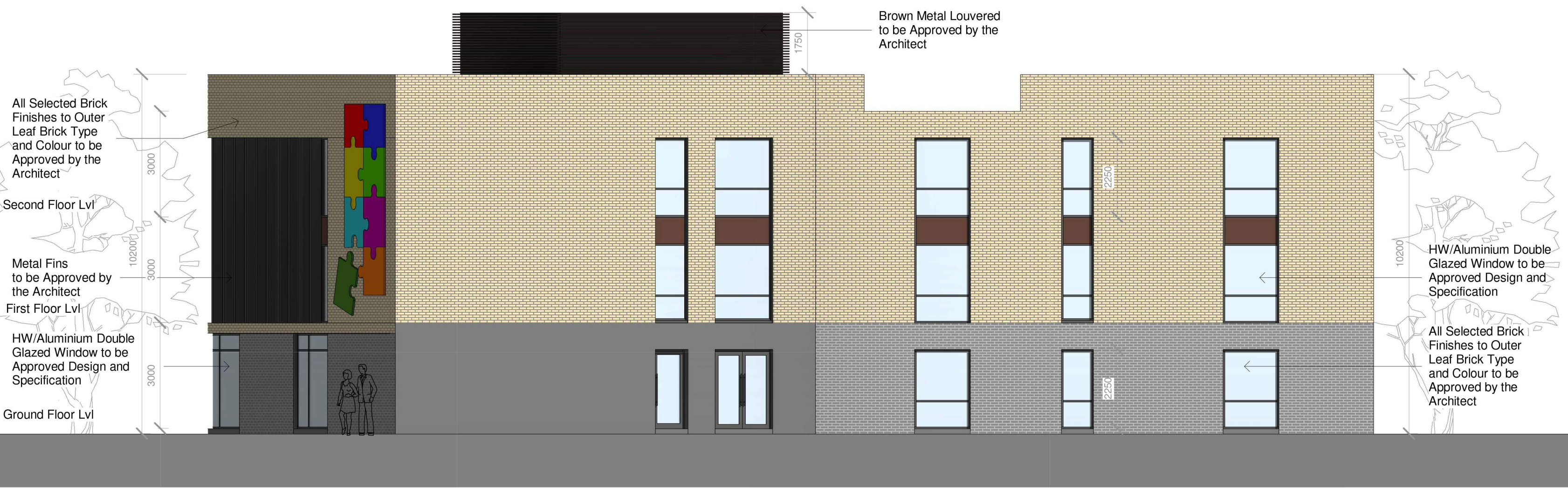
3 CRECHE-Rear Elevation (West) 1 : 100
