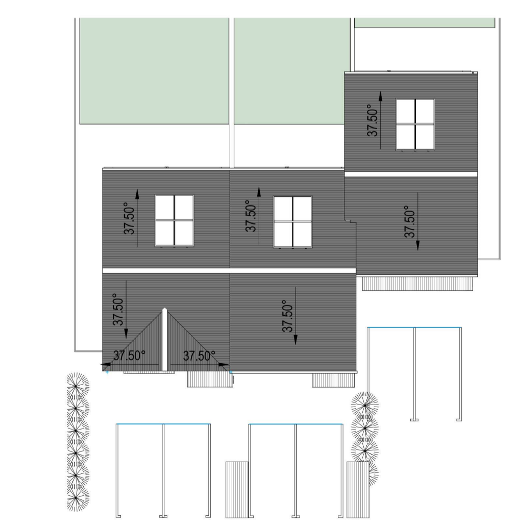
8 Block 3.2 - Roof Plan 1:200
