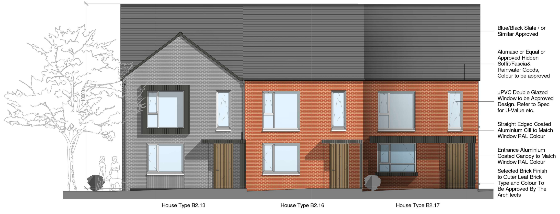
3 Block 3.2 - Front Elevation 1:100
