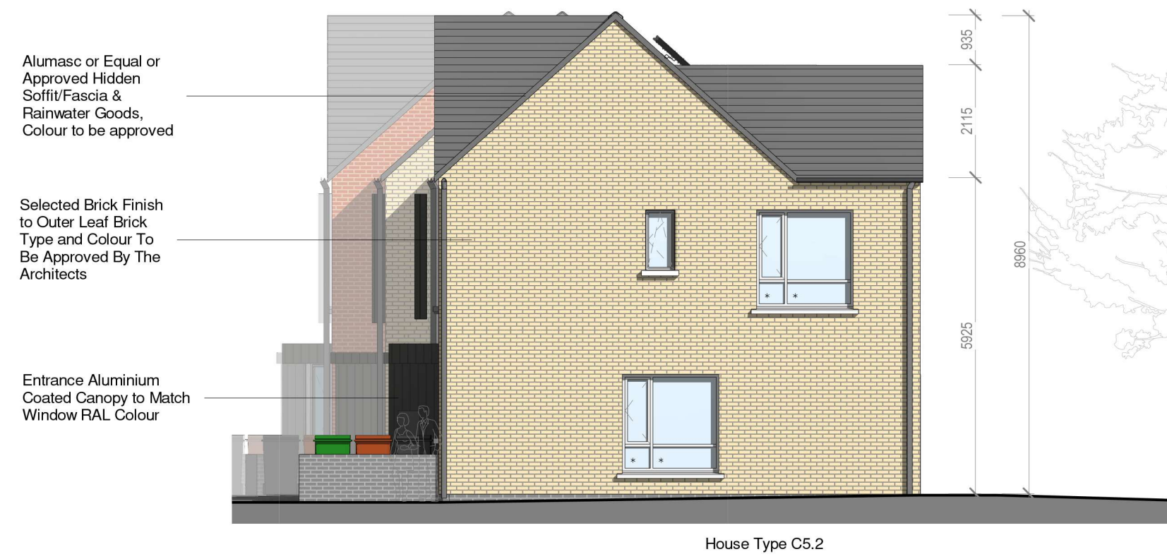
2 Block 5.5 - Side Elevation 2 1:100
