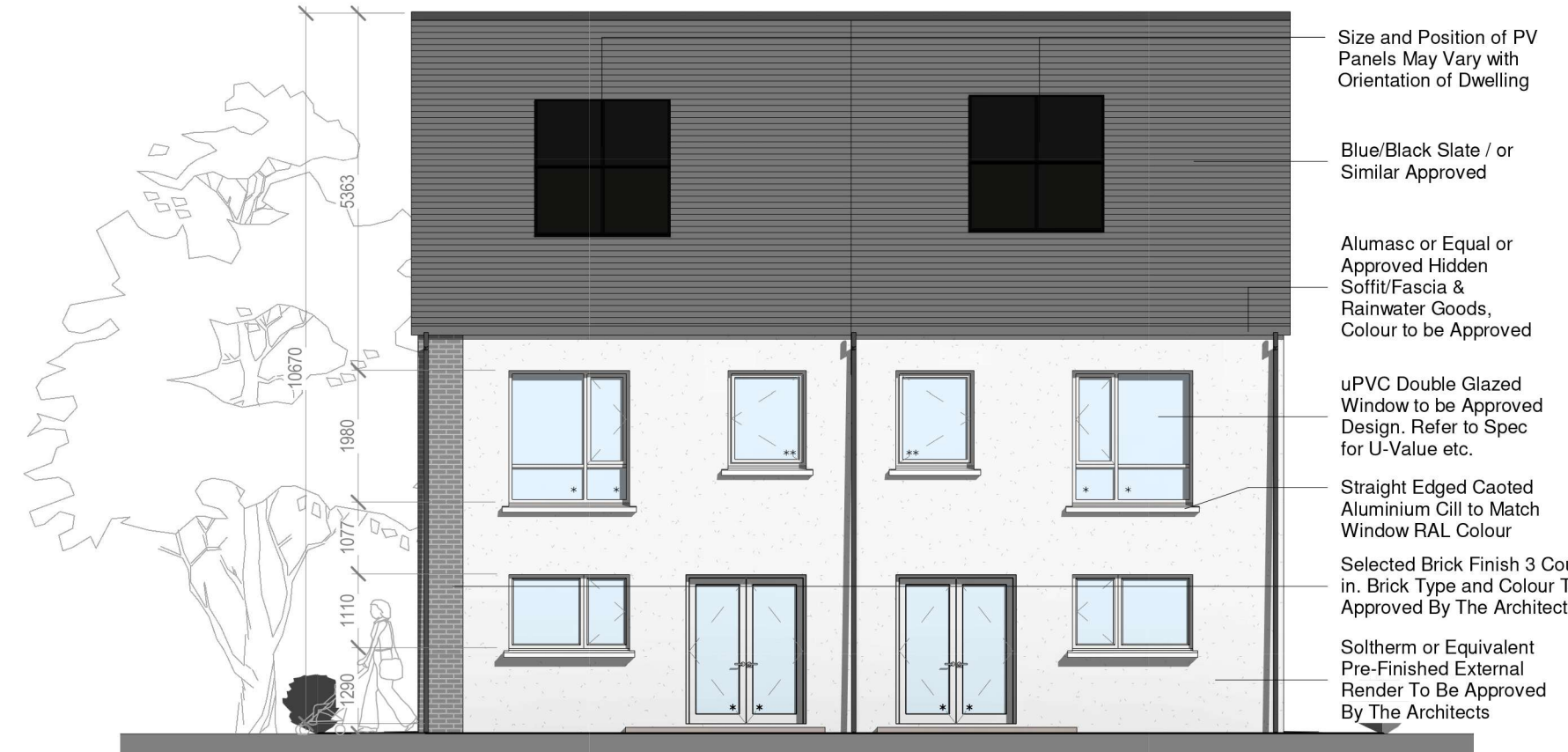
4 Block 7.1 - Rear Elevation 1:100
