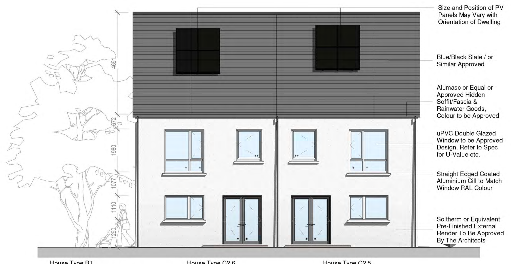
4 Block 7.2 - Rear Elevation 1 : 100
