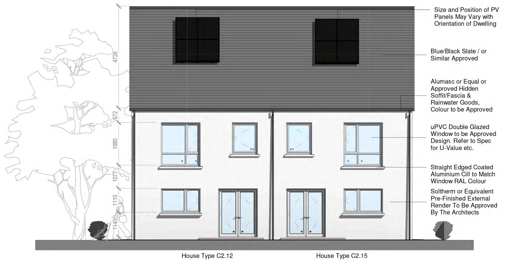
4 Block 7.3 - Rear Elevation 1 : 100
