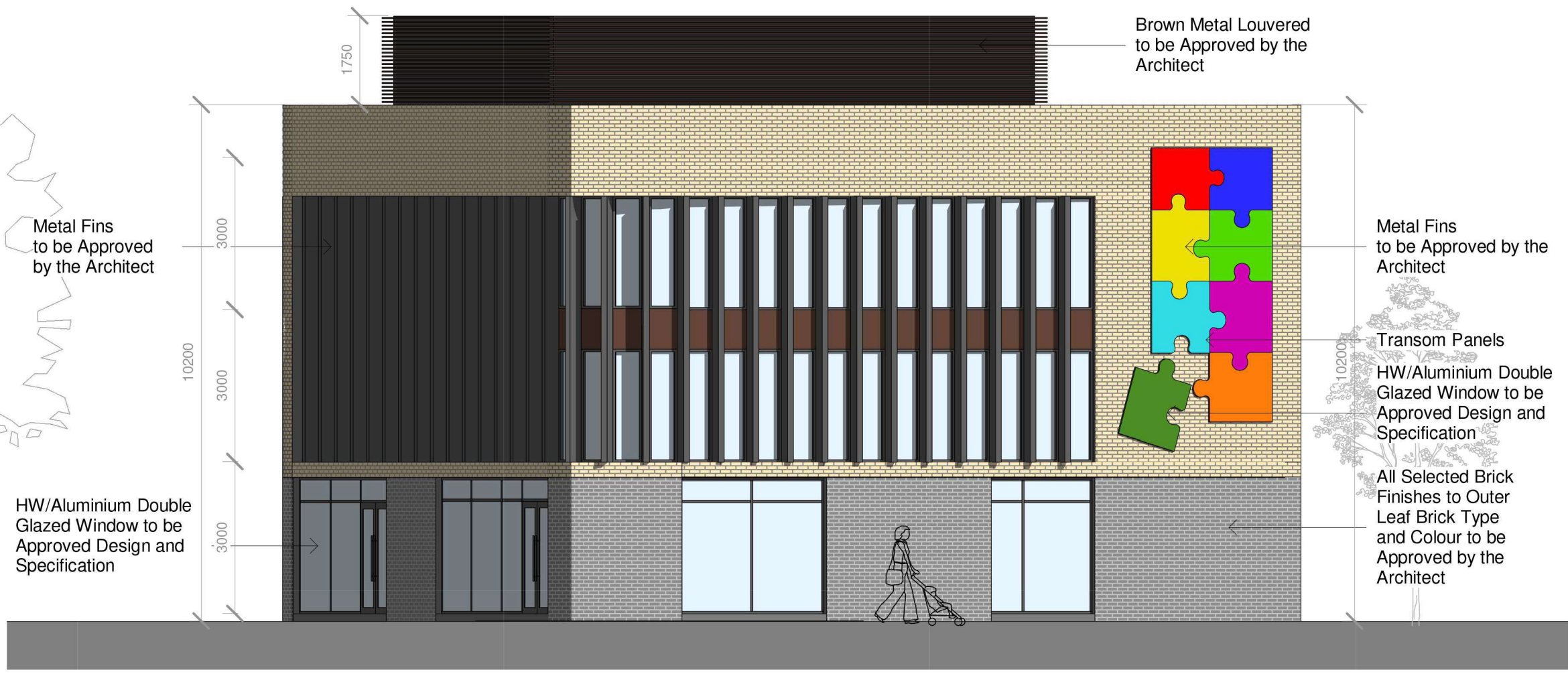
2 CRECHE-Side Elevation (North) 1 : 100
